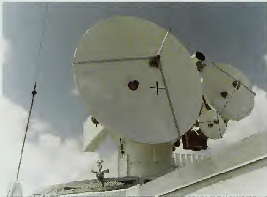
Fig. 6-17. The unmanned In-Flight Interceptor Communications data terminals are approximately 10 feet in height to include the 3-foot radome.
